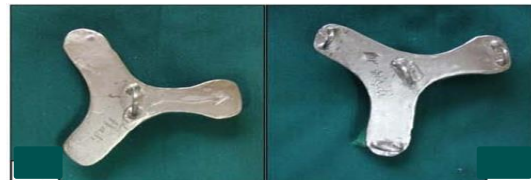
Figure 6- The Load cell transmitted the force from the machine to the overdenture
