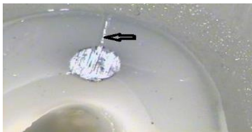
Figure 2- Horizontal view; the arrow shows the lateral crack perpendicular to the pin ( \times 25 )
