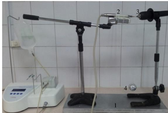
**Figure 1- Experimental design: (1) plate: (2) piezoelectric handpiece secured to arm: (3) manageable arm holding the implant: (4) 100 g pressure weight**
