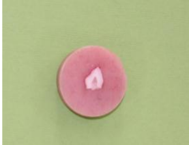
Figure 2- Sectioned and polished tooth embedded in acrylic resin
